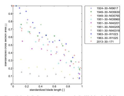
Figure 48: Standardised cross section versus standardised blade length of all objects.
