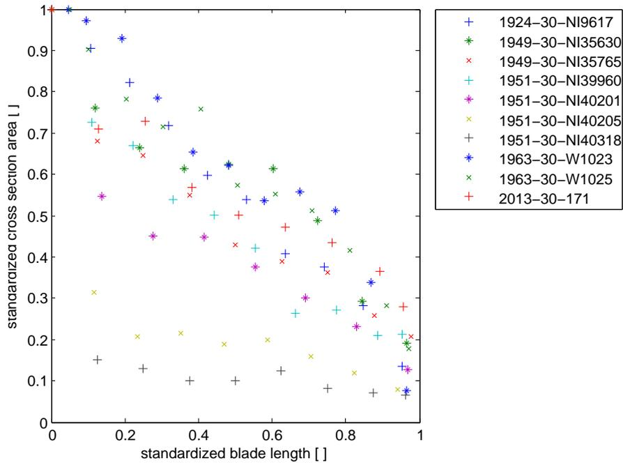
Figure 48: Standardised cross section versus standardised blade length of all objects.
