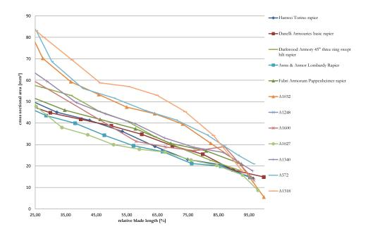
Figure 24: Cross section vs. relative blade length from 25% to point.
