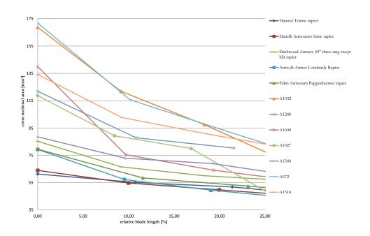
Figure 23: Cross section vs. relative blade length from hilt to 25%.
